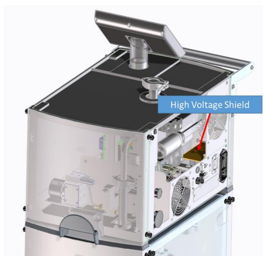
Figure 3: High Voltage Location
